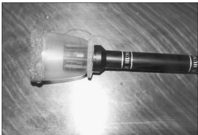
Fig. 1 - The closed chamber of the thermometry apparatus in which the handle of the infrared sensor is placed.
